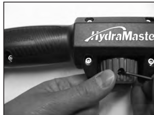
Figure 3-2. Remove Solution Control Knob
