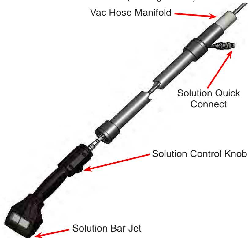
Figure 2-3. Attach Solution Hose and Adjust Water Volume
