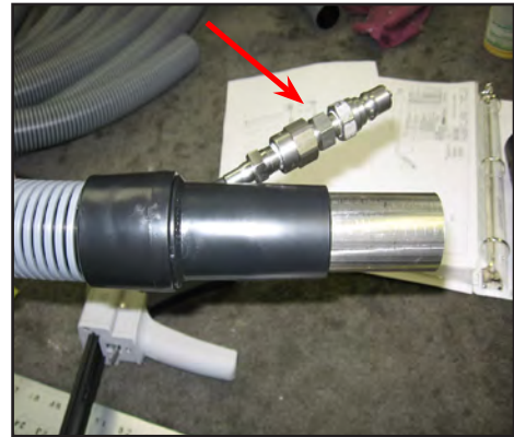
Figure 3-7. Disassemble Solution Quick Connect
