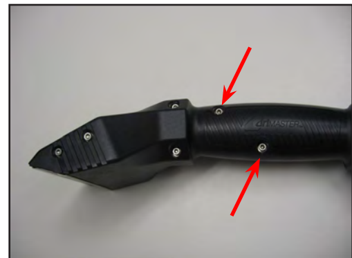
Figure 2-1. Remove Tool Screws
