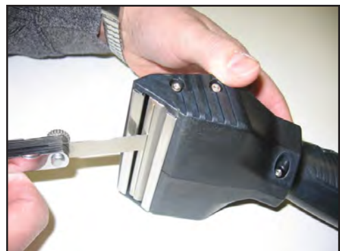
Figure 3-6. Clean the Solution Bar Jet
