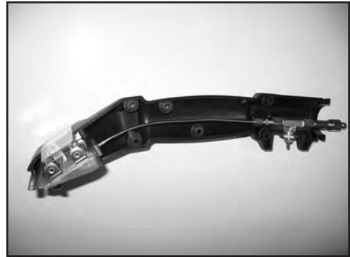
Figure 3-5. Re-install Clear Window Cover
